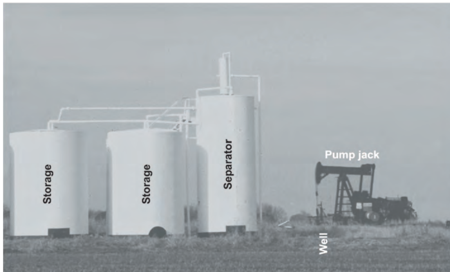
A typical oil well in Illinois. At the well head is the rocking pump jack (at the right). The oil-water mixture is pumped to the separator tank (center), and the oil then flows by gravity to one of the two storage tanks (left). The water flows to the other storage tank where it is collected and may be pumped back underground through an injection or disposal well. Photo by D. Morse.
